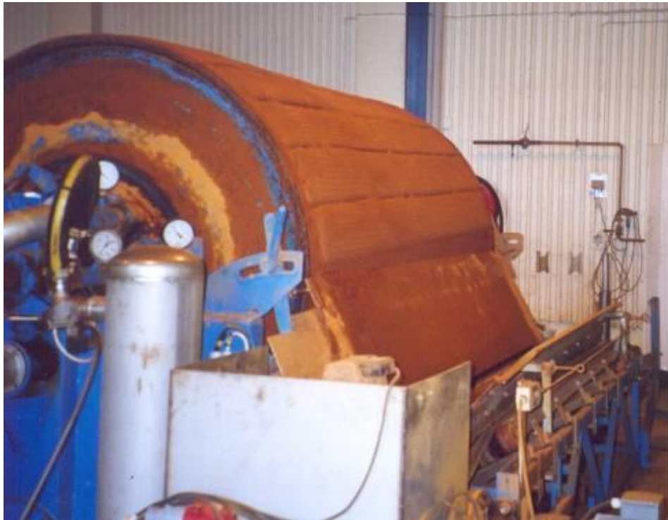
Figure 3: Drum vacuum filter dewatering metal hydroxide sludge from HDS processes at the Falun site, Sweden.
